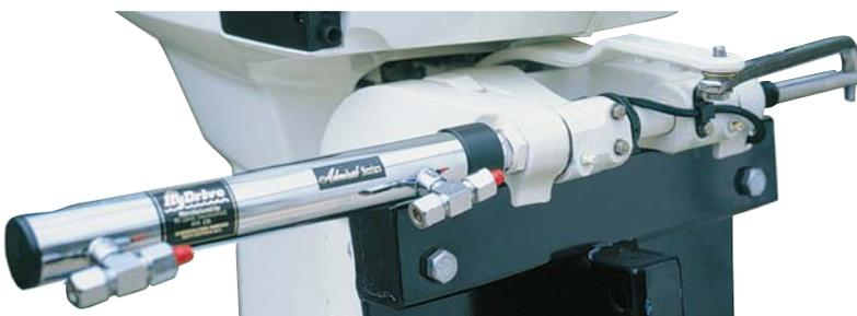
Like the 212T Sports cylinder above, the HyDrive 210T & 210TSE Tube-Mount cylinders are also designed for use on any brand STERNDRIVE (inboard/outboard) to replace conventional push-pull cable steering system. The cylinder screws directly to the bracket or pivot tube provided for the cable steering unit.
